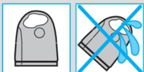
To prevent the cleaning fluid from leaking, ensure that the Clean&Renew station is placed on a flat surface. When a cleaning cartridge is installed, do not tip, move suddenly or transport the station in any way as cleaning fluid might spill out of the cartridge. Do not place the station inside a mirror cabinet, nor over a radiator, nor place it on a polished or lacquered surface.
