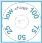
The shaver display ⑯ shows the charge status of the battery. During charging or when using the shaver, the respective green charge status will blink. When the battery is fully charged the green charge status will light up continuously, provided the shaver is switched on or connected to an electrical outlet.
